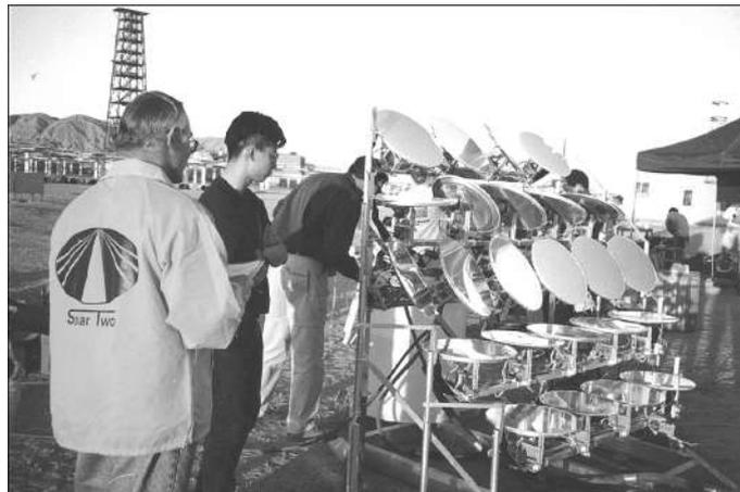
Fig 1. Stretched membrane concentrator cluster and focally positioned high temperature receiver.
