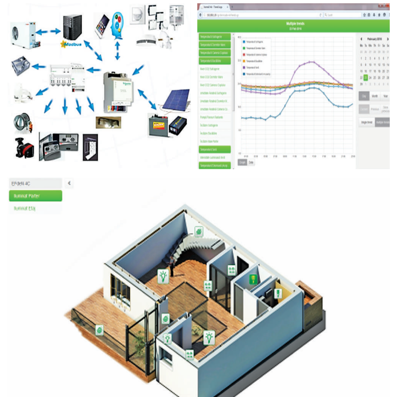
Fig.4. Equipment's integrated in the BMS system and monitoring interface
