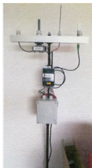
Fig. 3. Measuring tree with the devices CO 2 , and thermal comfort connected to the wireless network
